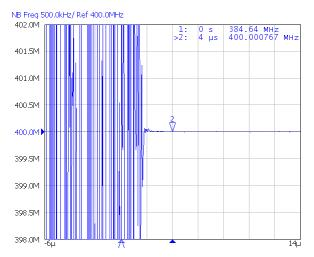
Figure 157. Buffer Power Up at 400-MHz Output
