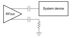
Figure 158. Unused Output Buffer Differential Pin
