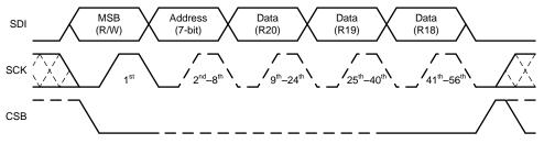
Figure 27. Block Programming Timing Example
