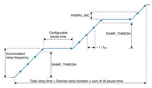
Figure 162. Auto Ramp Waveform
