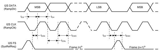
Figure 26. FSK I2S Timing Diagram
